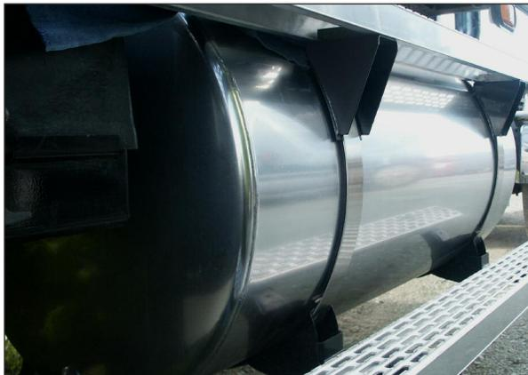
look. Next, it's important that the base coat is smooth and glossy since the Metallizing coat will mimic what's underneath. If the base coat is flat, the Metallizing coat will appear as a flat finish. If the base coat is semi-gloss, the Metallizing coat will appear as a semi-gloss finish. If special care is
